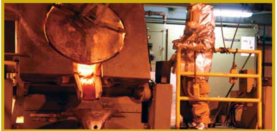
Top: A grinding circuit would pulverize the ore. Middle: Inside an autoclave where pressure oxidation takes place. Bottom: Refining the gold and pouring it into gold doré bars.
